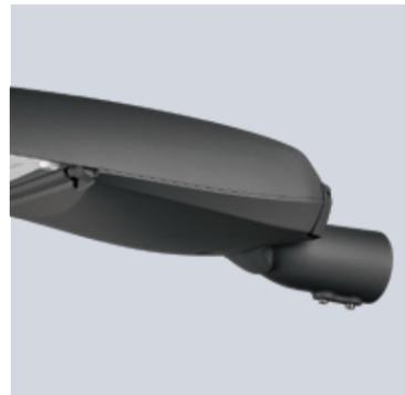
Horizontal or vertical pole mounting with Ø60mm spigot - Ø76mm bracket and Ø60-Ø42mm reducer accessory available.
