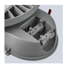
Specialist four bolt pole mounting mechanism allows fixing to Ø42mm to Ø60mm poles with a 5° adjustable angle.
